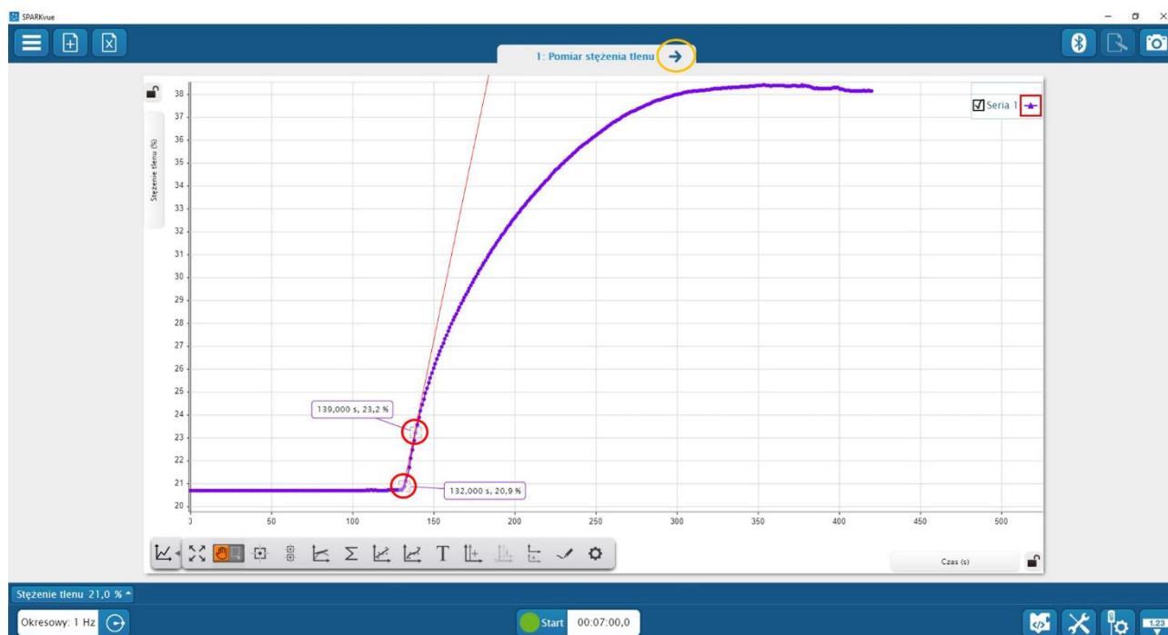
Fig. 10 Selection of measurements points required to determine the initial reaction rate.
