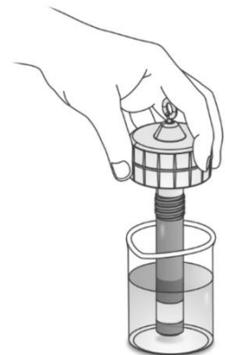
Figure 4. Oxygen sensor with metal part submerged in water.
